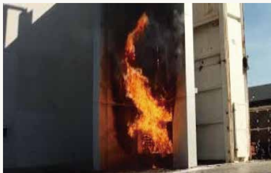
BS8414-1 (Fire-proof performance testing method for building exterior veneer system)
