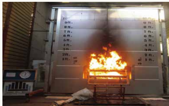
NFPA285 (Standard testing method for evaluating fire spread characteristics of non-bearing exterior walls containing flammable components)
